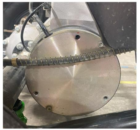
3) Once all 3 bolts have been removed, the EMB can be removed, exposing the gear and brake pad.
