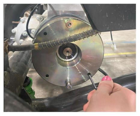
6) Align the splines of the gear with the 4 bolt EMB and work it on, tapping lightly with a mallet if necessary.
