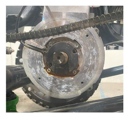
7) Install the new gear that was provided with your 4 Bolt EMB and secure it with the snap ring. You may need to tap it on with a mallet.
