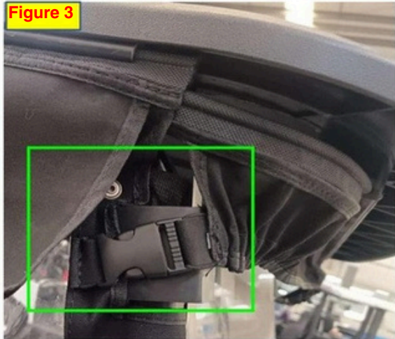
Step 2: Assemble the male and female plastic buckles: Insert the male buckle at the top of the front rain curtain into the female plastic buckles on the left and right sides of the rain curtain, referring to the green boxes and green arrows in Figures 2 and 3.
