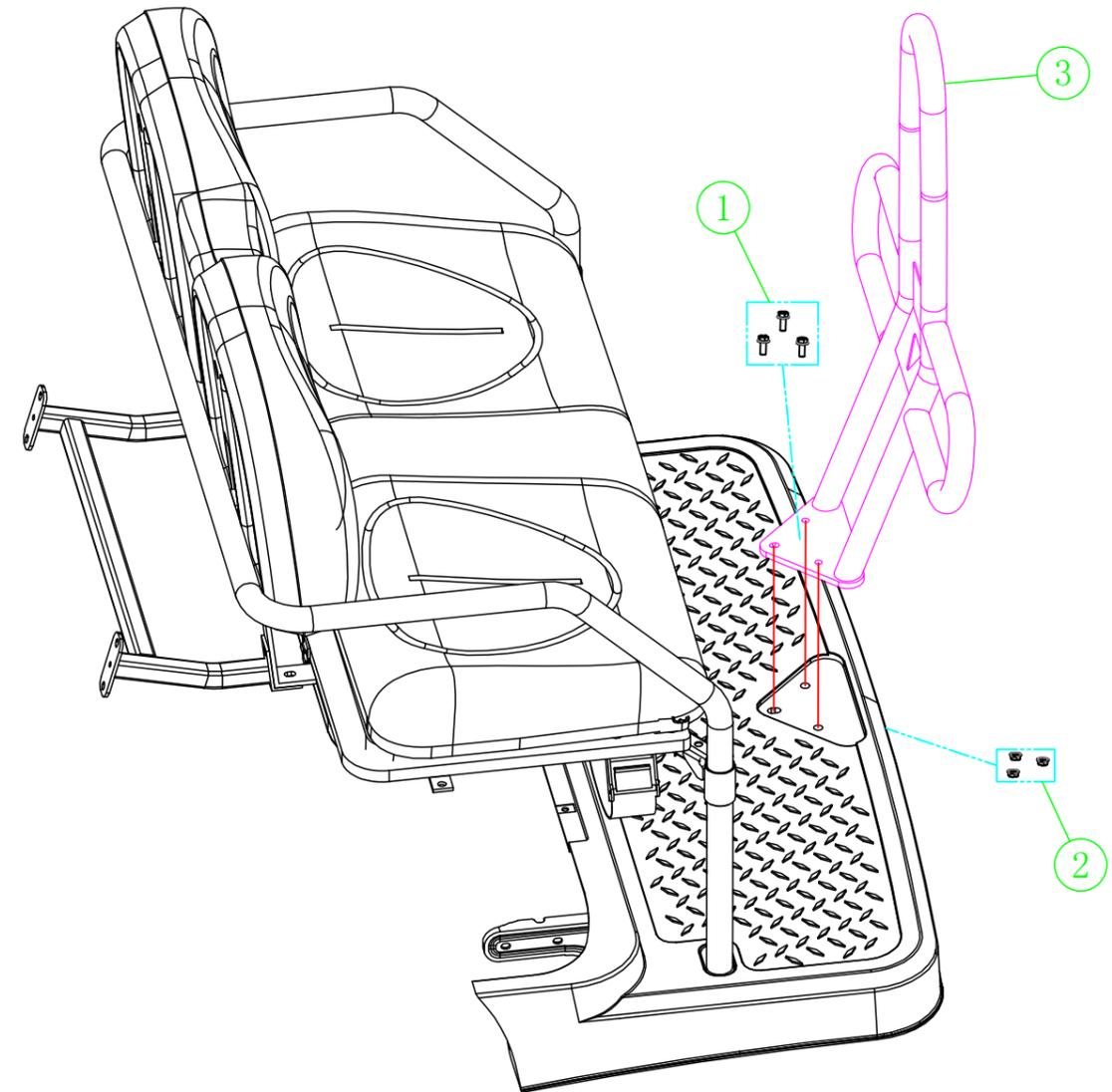
A617.2 assembly with flip golf seats, the top roof installation. (without rear seat and caddie plate )
