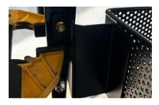
**Step 2**: Using a 8mm socket & drill, install one self-tapping on each side of the basket.
