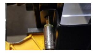
**Step 3**: Using a 8mm socket & drill, install the remaining self-tapping screws.
