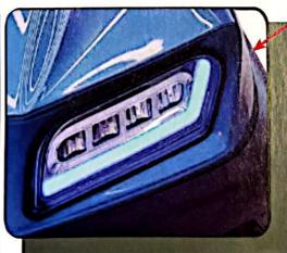
Insert this corner first, and then work the remaining trim ring around head-light and snap into body.
