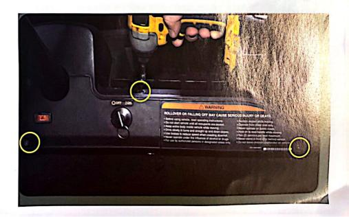
Find a desired location on your dash to mount the hazard switch. Keep in mind you will need a location for USB in Step 11 also. Ensure the location is free of and will not affect dash reattachment. Using a 15/32" drill bit, drill a mounting hole and insert switch into dash. Secure with the ring nut from back of switch.
