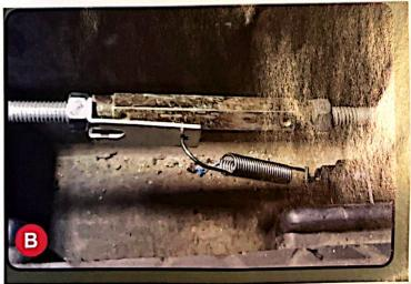
Plug the two bullet connectors from the brake switch into the corresponding connectors on the wiring harness. Secure all wiring so that it is out of the way of the brake components.
