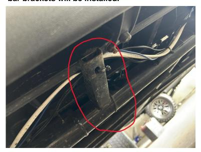
Step 2: Hold the bracket flush to the frame and use a center punch or marker to mark 4 holes per side as shown.
