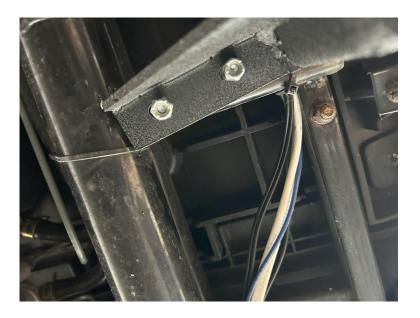
Step 7: Double-check all alignment. Once satisfied, fully tighten all hardware on both sides.
