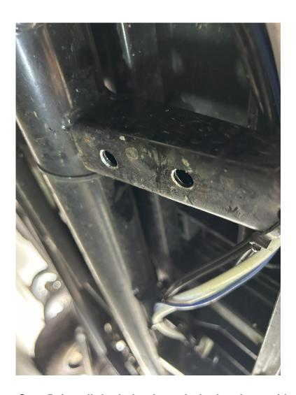
Step 5: Install the bolts through the bracket and loosely secure with nuts on the underside. Do not fully tighten yet.
