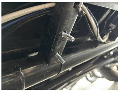
Step 6: With brackets loosely in place, align the nerf bar step and begin securing it to both mounting brackets.
