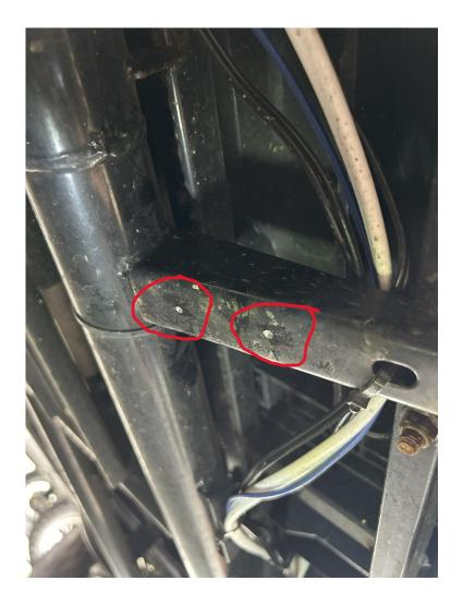
Step 4: Drop the provided bolts from the top down through the holes you've drilled.
